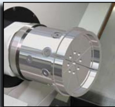
Multiple OD Gripping Locations with Independent Travels
